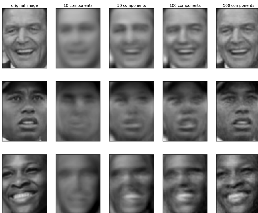
Figure 3-11. Reconstructing three face images using increasing numbers of principal components
